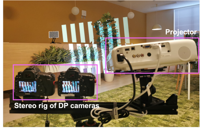
Fig. 6: Our DP structured-light stereo setup.
